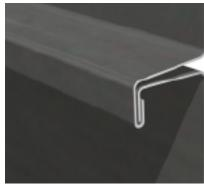
Vertical and horizontal standingseam joint
